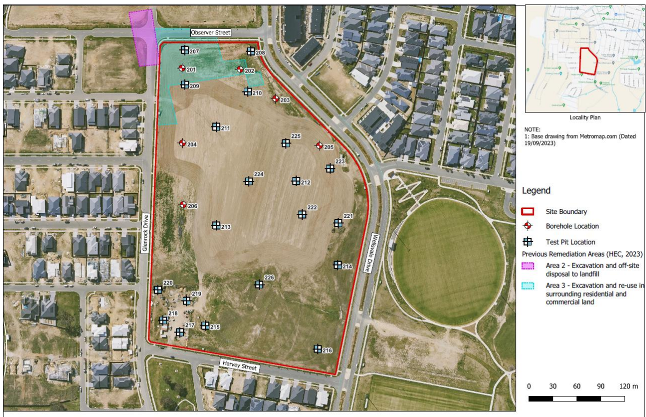
Figure 30: Previously excavated areas and locations of DSI boreholes and test pits
